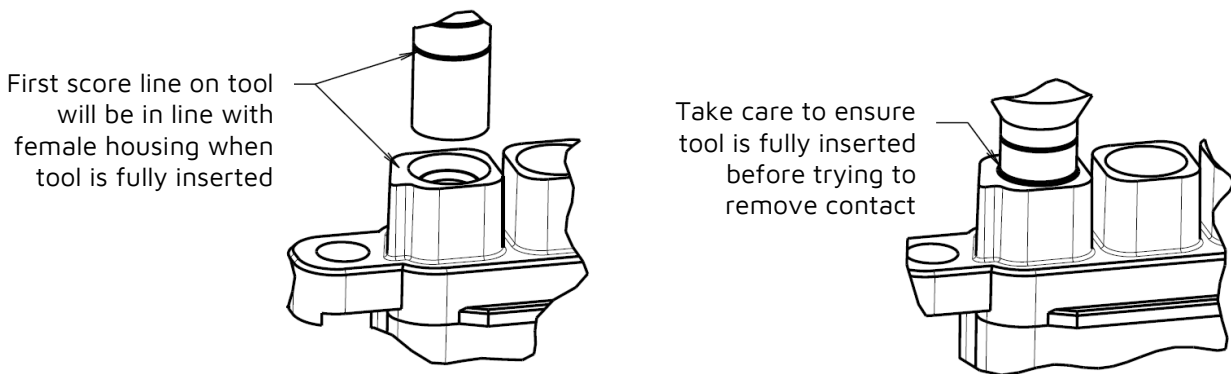
Figure J: Female Contact Removal
