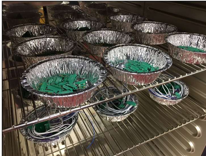
Individual connectors and mated assemblies in the oven for 96, 250 and 1,000 hours
