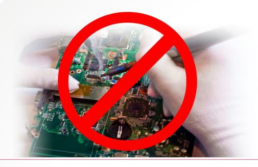
Hand-soldering the can to the PCB increases the risk of localized hot-spots during this operation. Those hot-spots could damage other components, especially any devices more sensitive to heat.
