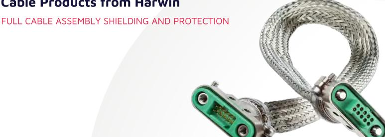
In combination with the metal backshells, adding metal braiding along the length of the cable assembly completely shields the whole product. We can supply a fully finished cable assembly with the shielding braid fixed in place with Band-It ties. For the Gecko-SL product range, we have even developed a standard part numbering system for these options.
