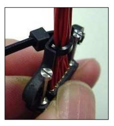
5. Fit the second Cable Hood housing. Use a No.1 Pozidriv screwdriver to assemble the two retaining screws (one in each side of the hood). Tighten the retaining screws to a torque of 18Ncm. **DO NOT OVER-TIGHTEN.**
